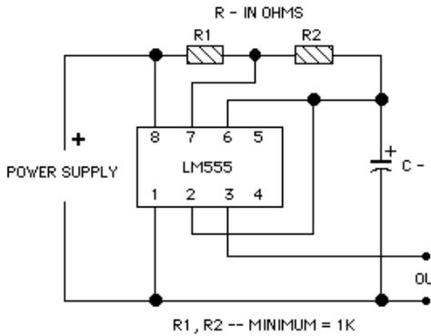
TO CALCULATE THE FREQUENCY --  $F = \frac{1}{0.693 \times (R1 + 2 \times R2) \times C}$
