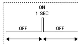
CIRCUIT WILL TIME OUT EVEN IF THE TRIGGER IS HELD CLOSED
