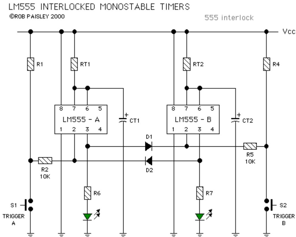
PREVENTS SECOND TIMER FROM BEING TRIGGERED WHILE THE FIRST IS RUNNING
