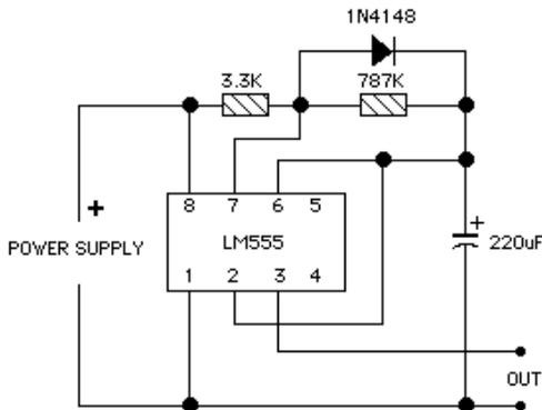
DUE TO THE DIODE IN THE TIMING CIRCUIT THE ABOVE FORMULAS DO NOT WORK DIRECTLY
