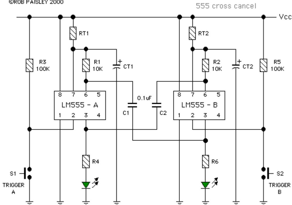
TIMERS RESET EACH OTHER WHEN AN "OFF" TIMER IS TRIGGERED
