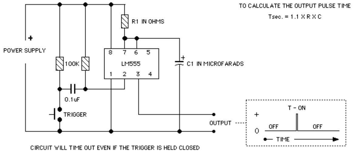
CIRCUIT WILL TIME OUT EVEN IF THE TRIGGER IS HELD CLOSED
